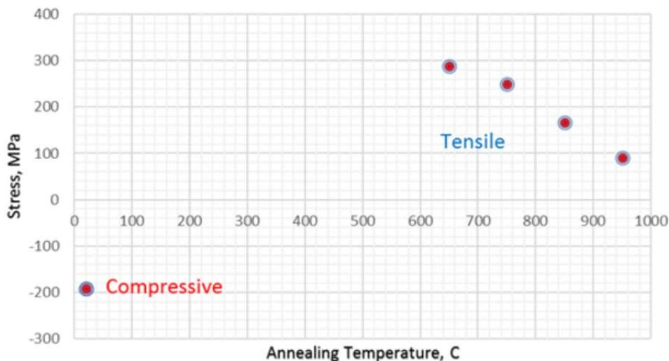
**Fig. 1.** Measured stress in nc-Si films annealed at different temperatures. The compressive stress of the original amorphous film changes to tensile by annealing and the tensile stress decreases as a function of the annealing temperature. The annealing time was 60 minutes for all the wafers.
