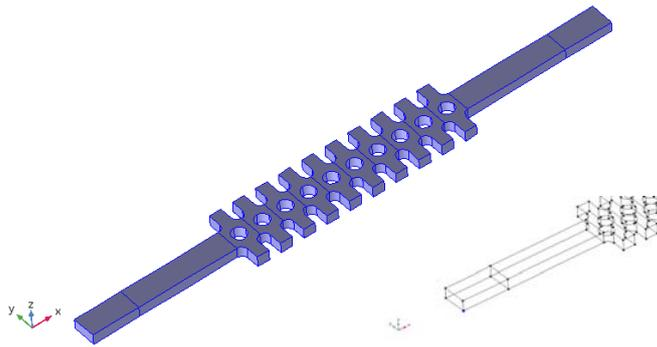
**Fig. 9.** Geometry of a 3D nanobeam model. The inset displays one of the two points where  $y$ - and  $z$ -displacements are set to vanish.
