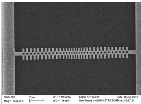
**Fig. 3.** SEM image of a one-dimensional optomechanical cavity made of nc-Si annealed at 950 C. The thickness of the beam is 212 nm.
