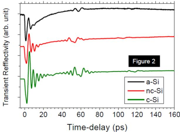
**Fig. 2.** Time-of-flight scans measured from amorphous, nanocrystalline and crystalline (100) silicon. The measurements show that the sound velocity in nc-Si is higher than in (100) c-Si.
