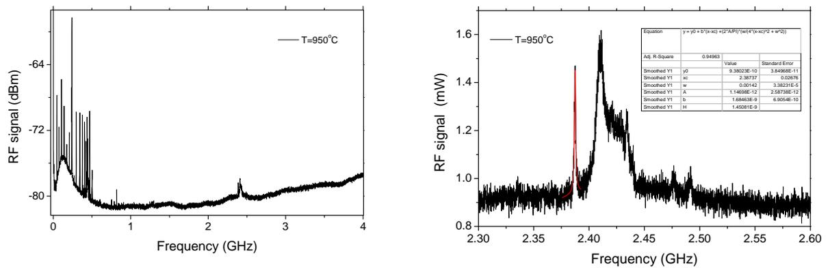
**Fig. 7.** (Left) RF spectrum of an OMC made of nc-Si annealed at 950 C. (Right) Zoom of the spectrum around 2.45 GHz.
