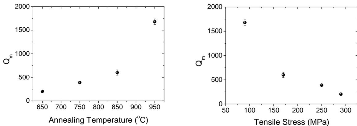
**Fig. 8.** (Left) Mechanical Q-factor as a function of the annealing temperature of the nc-Si film. (Right) Mechanical Q factor as a function of the tensile stress.
