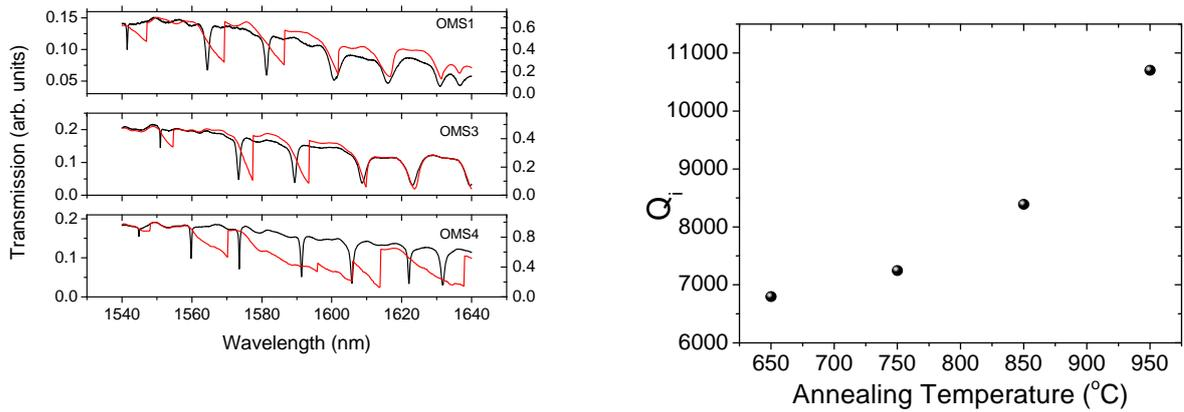
**Fig. 5.** (Left) Optical transmission spectra at low and high intracavity photon number (black and red curves respectively). (Right) Optical Q-factor as a function of the annealing temperature.
