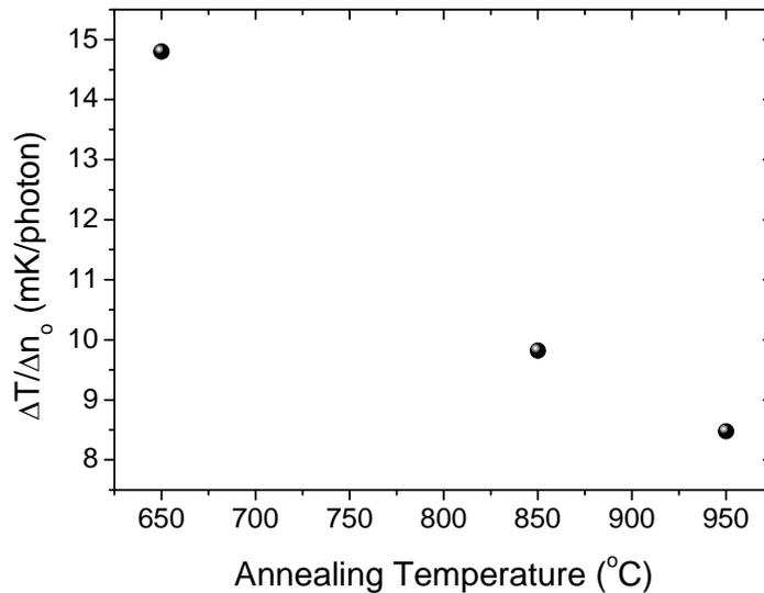
**Fig. 6.** Effective temperature increase of the cavity per photon as a function of the annealing temperature of the nc-Si film.
